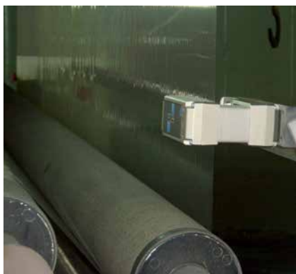
Ultrasonic edge sensor FX 5 in film manufacturing machine
