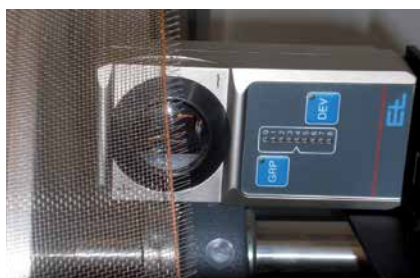
Infrared edge sensor FR 52 for mesh acquisition
