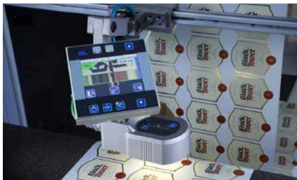
Color line sensor FE 52 on roller inspection machine
